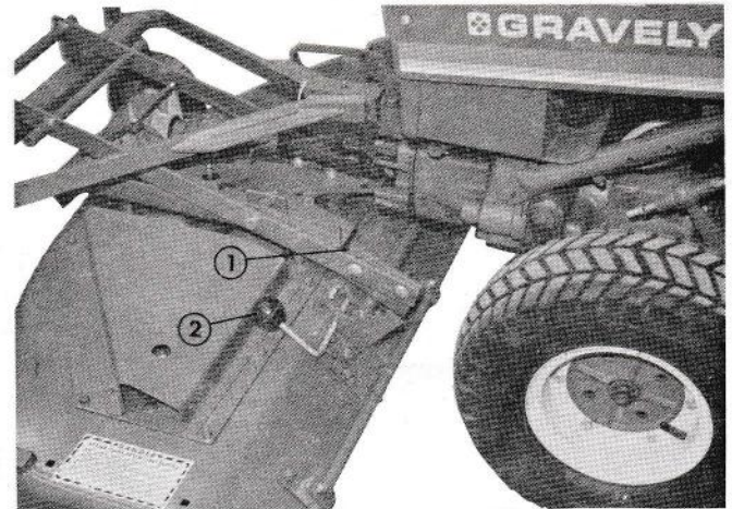
1 - Adjusting Cam 2 - Height Adjustment Lever
